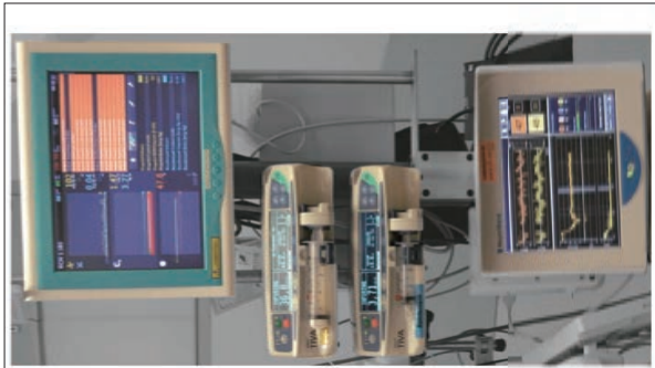
Figure 1. Control-RP system with touch-screen user interface (top) connected to a patient in an operating room (bottom) with the corresponding hardware and NeuroSENSE (BIS) and Bispectral Index.
